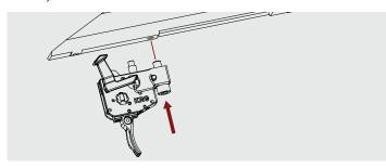
Step 3: Install barreled action back into stock.
