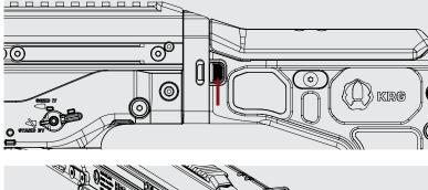
**Step 2:** Push this button to unfold the stock. The latch mechanism to hold the buttstock in the folded position is a positive lock system. You MUST press the unlock button pictured above to unfold the stock. It does not release just by pulling on the buttstock.
