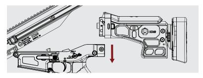
**Step 2:** Close the breech area then push the upper and lower detent pins back into place.
