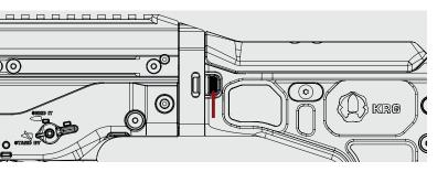
NOTE: Retighten the brass set screw inside the latch mechanism if your folding action feels loose.
