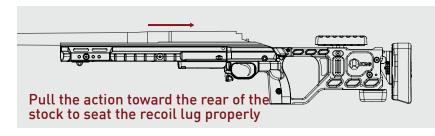
**Step 5:** Making sure the action is level and not canted to the left or right, next tighten all three action screws until they are snug but not fully tightened.
