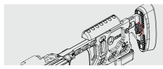
Step 2: Slide the buttpad up or down in 1/4" increments, or cant it 15 degrees to either side. There are protrusions on the aluminum LOP bar that fit into pockets on the polymer buttpad housing. Retighten Thumbscrew when you have it set where you want.
