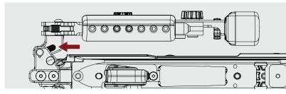
**NOTE:** The latch mechanism to hold the buttstock in the folded position is a positive lock system. You MUST press the unlock button pictured above to unfold the stock. It does not release just by pulling on the buttstock.
