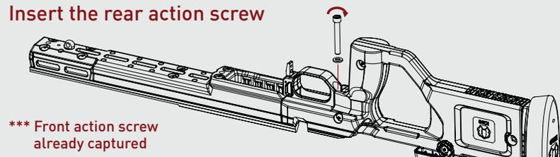
**Step 3:** Pull the action towards the rear of the stock while holding the stock stationary. This is to seat the action against the recoil lug. A good way is to set the rifle vertical on the butt pad and bounce it lightly on the ground a couple times.
