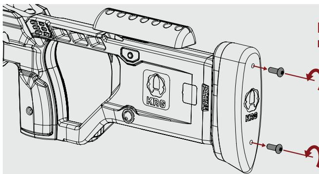
**Step 2:** Replace these screws with the longer screws, which are long enough to go through your desired amount of spacers. Insert desired quantity of spacers onto the longer screws
