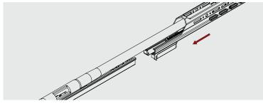
**Step 4:** Insert and tighten new forend screws included with Arca Rail Enclosed Forend. Use the 6x button head M5 x 25mm screws at the front and the 2x button head M5 x 40mm screws through the magwell.
