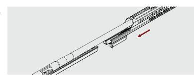
Step 3: Insert and tighten included forend screws. Use the 6x Button Head M5 x 25mm screws.
