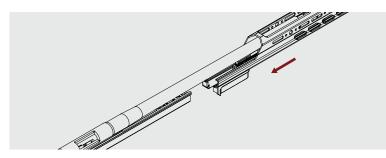
**Step 4:** Insert and tighten new forend screws included with Arca Rail Enclosed Forend. Use the **6x Button Head M5 x 25mm** screws at the front.
