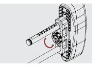
Step 2: Slide the buttpad up or down in 1/4" increments, or cant it 15 degrees to either side. There are protrusions on the aluminum LOP housing that fit into pockets on the polymer buttpad housing. Retighten Thumbscrew when you have it set where you want.
