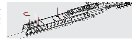
Step 2: Slide the forend forward or backward a small amount to achieve the desired fit of the magazine into the stock. Re-tighten screws from step 1.
