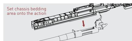
**Step 3:** Drop the rear action screw into the hole just behind the trigger guard, turn the screw to engage the threads in the action. Again do not fully tighten.
