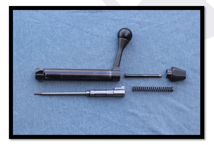
The TRG firing pin assembly is composed of three machined parts plus the spring. The firing pin itself is a simple turned part with a rounded tip of about .068" (1.7mm) in diameter. The tip is discolored from hardening while the body does not show similar discoloration. It may
