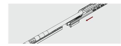
Step 4: Insert and tighten new forend screws included with Enclosed Forend.
