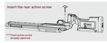
**Step 3:** Pull the action towards the rear of the chassis while holding the chassis stationary. This is to seat the action against the recoil lug. A proven method is to place the rifle upright, resting on the buttpad and lightly bounce it on the ground two to three times.
