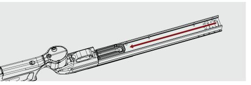
Step 4: Reinstall the chassis forend and install the barrelled action into the chassis. Torque action screws to spec.
