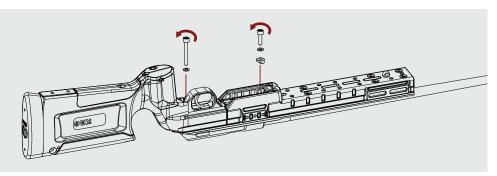
**Step 2:** Separate the polymer forend from the aluminum backbone by first removing the **8 forend screws** using a **3mm hex key**. Then, pull the forend by the mag well end, away from the chassis.
