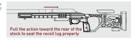
**Step 5:** Making sure the action is level and not canted to the left or right, next tighten both action screws until they are snug but not fully tightened.
