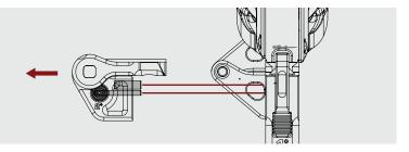
Step 3: Using a 2.5mm hex bit, remove the four M4x12mm flat head screws in order to remove the bottom hinge.
