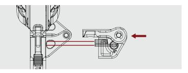
**Step 6:** Apply a small amount of blue Loctite to the **M6x25mm button head screw** and **M6x18mm flat head screw** and attach top hinge to the chassis.
