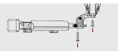
**Step 2:** Remove the top hinge, ensuring both pins remain inside the hinge. The smaller-diameter pin secures the secondary release button in place and should not be removed.
