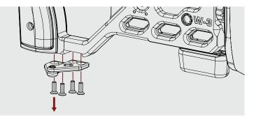
Step 4: Reverse the bottom hinge to the oposite side and retightened the four M4 x 12mm flat head screw. Tighten to 45 in-lbs.
