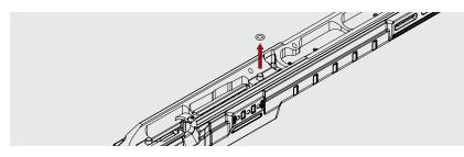
**Step 2:** With the chassis upside down, set chassis' bedding area (V-block for Tikka and Radiused area for Remington) onto the action. Using a 5mm or 3/16" hex bit (depending on inlet), turn the front action screw to engage the threads in the action to draw the action into the chassis, do not fully tighten at this point.
