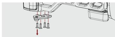
**Step 4:** Reverse the bottom hinge to the oposite side and retightened the four M4 x 12mm flat head screw. Tighten to 45 in-lbs.
