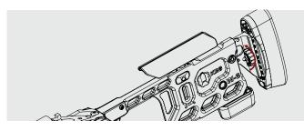
**Step 2:** Slide the buttpad up or down in 1/4" increments, or cant it 15 degrees to either side. There are protrusions on the aluminum LOP bar that fit into pockets on the polymer buttpad housing, assuring positive lock up. Retighten Thumbscrew when desired position is achieved.
