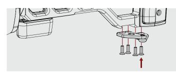
**Step 5:** Reverse the top hinge and reinsert into the chassis. The release button will move to the bottom of the hinge.
