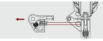
**Step 3:** Using a 2.5mm hex bit, remove the **four M4x12mm flat head screws** in order to remove the bottom hinge.
