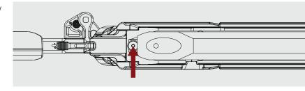
**Step 3:** Tighten action screw to your preferred torque level. Sako has not put out an official figure for the torque value so we default to 45-65 in-lbs.
