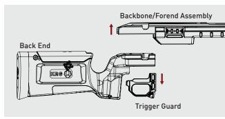
Step 2: With a 3mm hex bit, install the trigger guard to the Pro Front End using the included M5x10mm low-profile screw.
