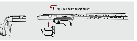
Step 3: Slide down the Pro Front End onto the Back End until it makes positive contact with the rear abutment.
